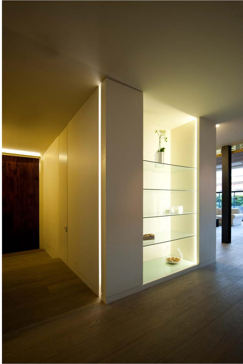
the minimal sculpture display area with concealed lighting slot detail, illuminating the concealed cloak room. the right hand side of the display opens as one huge hidden door to access and change the light bulbs
